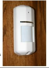
Installation: For best results install the XC-1XT at a mounting height between 6.6 ft (2.4m) and 8.2 ft (2.5m). Mount the unit so it is looking into an area free of obstructions, do not mount the unit so it is looking directly at heating or cooling sources. Avoid viewing operating machinery or objects which have the potential for movement. Do not aim unit so it is looking at public road/pathways.
