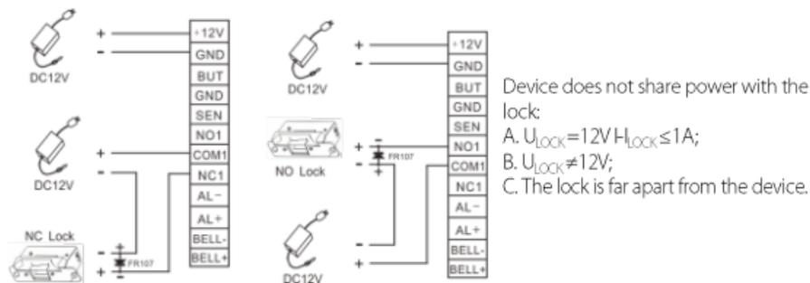
$I$ : device output current,  $U_{LOCK}$ : lock voltage,  $I_{LOCK}$ : lock current.
